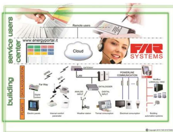
Figure : The FAREcho "Energy Portal" and its interface with ICT system components
